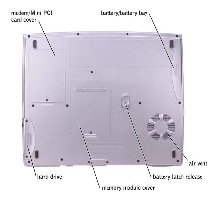
MODEM/MINI PCI CARD COVER — Covers the compartment that contains the modem and Mini PCI card. See page 103.
