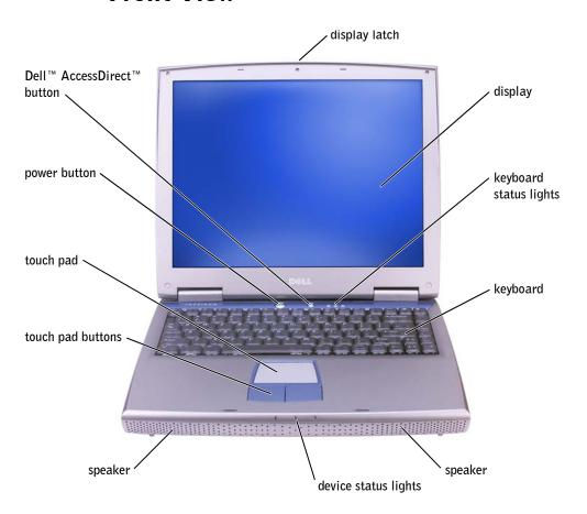
**DISPLAY LATCH** — Keeps the display closed.
