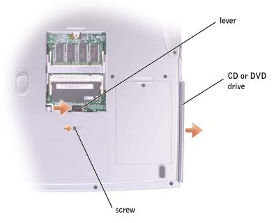
**4** Press the lever next to the memory module connectors in the direction of the arrow on the lever (towards the drive) to release the drive.
