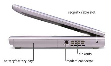
**BATTERY/BATTERY BAY** — When a battery is installed, you can use the computer without connecting the computer to an electrical outlet. See page 41.
