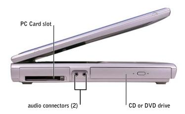
**PC CARD SLOT** — Supports one PC Card, such as a modem or network adapter. For more information, see "Using PC Cards" in the Tell Me How help file. To access the help file, see page 80.
